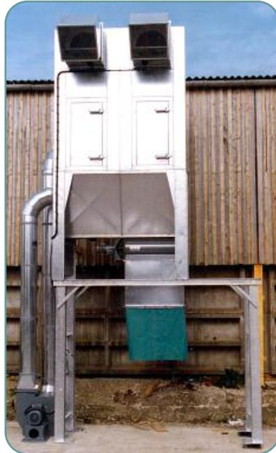
**Filter/Collector type "Bagging unit":** A "Duplex" twin bag filter/collector unit, suitable for indoor use only, with an integral fan/motor. This type of unit can be fitted with fans from 1.5kW to 7.5kW and up to four collection bags. A simple and low cost system suitable for joinery and similar applications. The size of filter sleeves can be increased in length to provide a low filtration velocity to suit different materials/applications.
